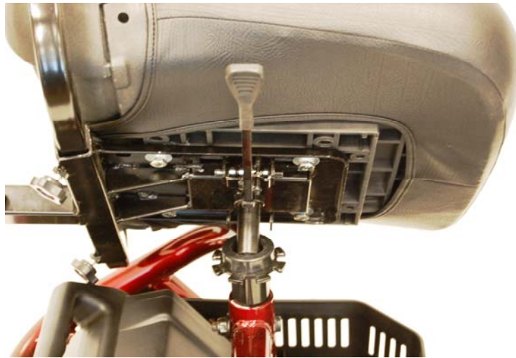
Figure 23. Installing the Seat
