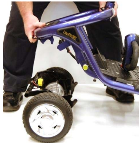
Figure 18. Lifting the Frame
